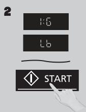
The oven automatically defaults to the imperial measure system (oz/lb). Press Start to cycle between the weight system, Metric(g/kg) or Imperial (oz/lb)
