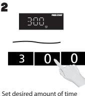
Set desired amount of time using **Number** pads (up to 99 minutes, 99 seconds).
