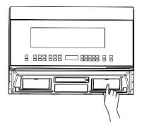
Removing and Cleaning the Filters
