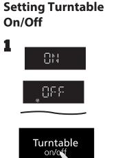
For best cooking results, leave the turntable on. It can be turned off for large dishes. Press **Turntable On/Off** pad to turn the turntable on or off. When you turn it off, on or off. will appear in the display window.
