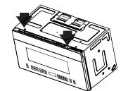
Remove 2 grille screws to remove the grille.
