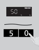
Enter the desired weight by pressing number pads. The weight is 0.1-6.0 Lbs.
