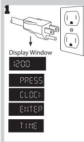
Plug into a properly grounded electrical outlet. "12:00 PRESS CLOCK ENTER TIME " message scrolls across display window.
