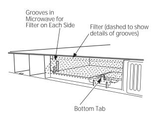
*To Install the Charcoal Filter To install a new charcoal filter,* remove plastic and other outer wrapping from the new filter.
